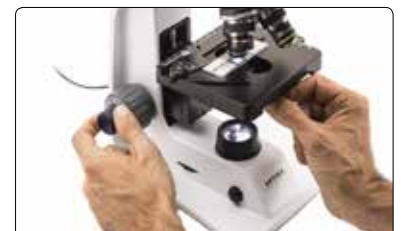
Regulation of diaphragm aperture
