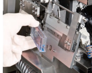
Installation of the cassette
